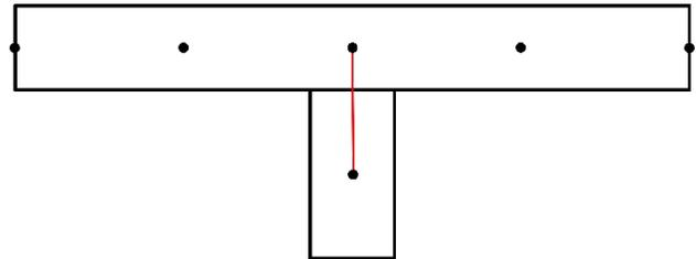
Fig. 4. T-beam modelled with a combination of beam and shell elements. The beam elements are moved vertically and connected with rigid links.
