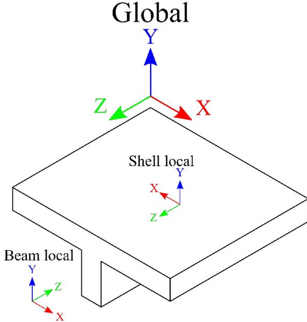
Fig. 5. Axis orientation used to construct the following equations.
