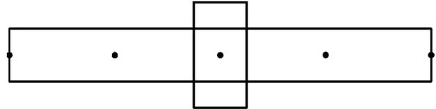
Fig. 3. T-beam modelled with a combination of beam and shell elements—no offset.
