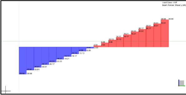
Fig. 6. Beam: Shear force in the beam ( $V_{beam}$ )
